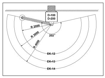
• D-100 and D-200 filter units are usually used with extraction arms. The dimensions of the standard VANTERM arms are given below:
