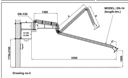
The extraction arms can be used together with DK-150 extension crane to increase the working range of D-100 and D-200 filter units. The working ranges of D-100 and D-200 are shown in the drawings above.
